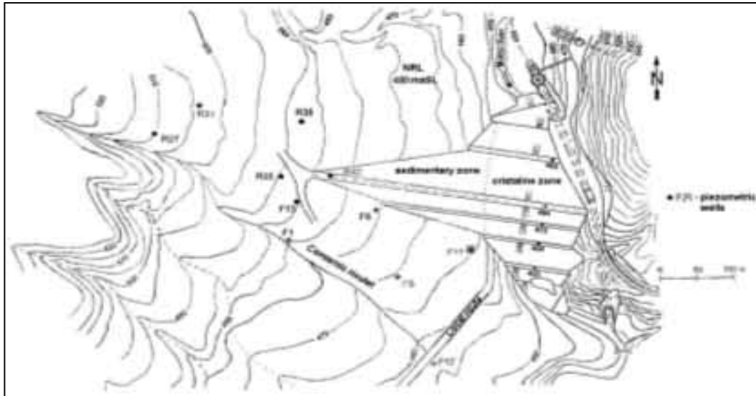
Figure 3 Location of some piezometric wells at Motru dam
