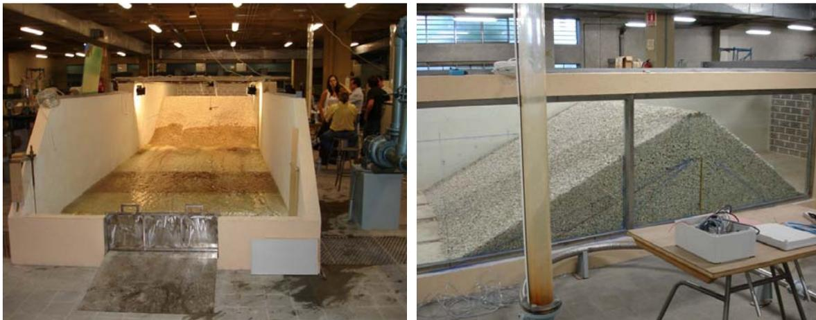
Figure 5. Case A. Some photos of the experimental channel and of and homogeneous dam
