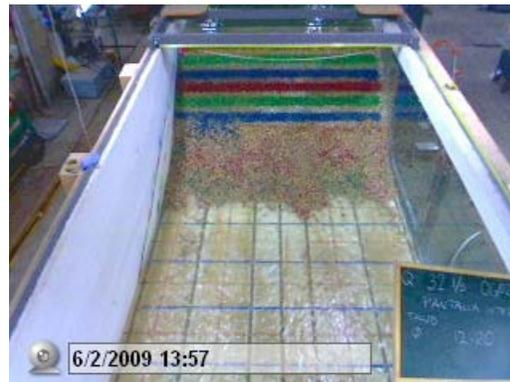
Figure 11. Case B.2.2 Steady state stable configuration achieved for a discharge  $Q_{B22}$ .
