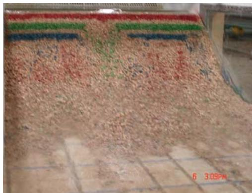
Figure 12. Case B.2.3 Steady state stable configuration achieved for a discharge  $Q_{B23}$ .
