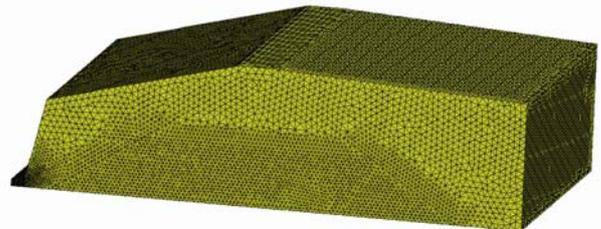
Figure 5. Case A1. 3d mesh. 1.260.000 linear tetrahedral elements.
