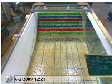
a) Experimental length of failure  $B_{exp} = 0.32m$
