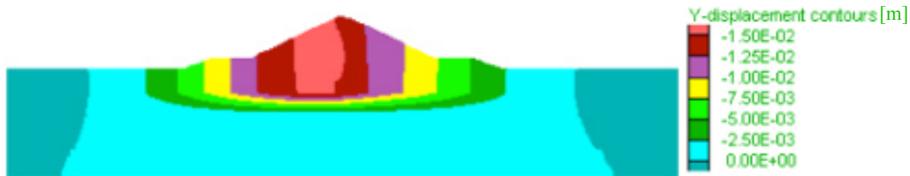
Vertical displacements [m] after the degradation of the first layer from Step 1 to Step 11
