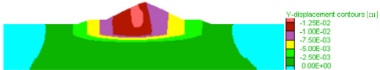
Vertical displacements [m] after the degradation of the first layer from GSI=80 to GSI=15
