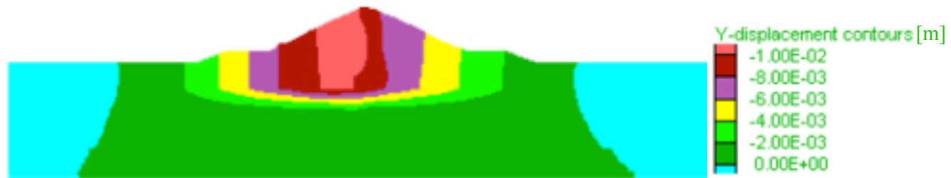
Vertical displacements [m] after the degradation of the first layer from GSI=80 to GSI=10
