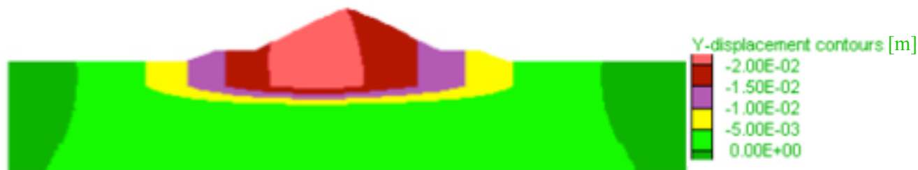
Vertical displacements [m] after the degradation of the first layer from Step 3 to Step 13
