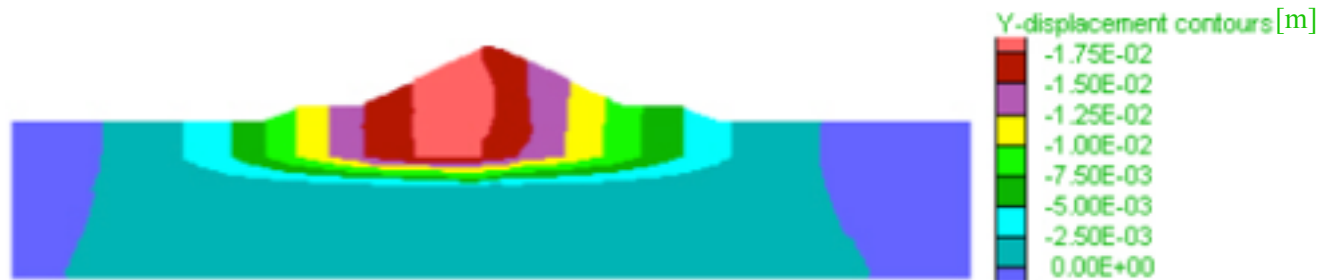
Vertical displacements [m] after the degradation of the first layer from GSI=50 to GSI=10
