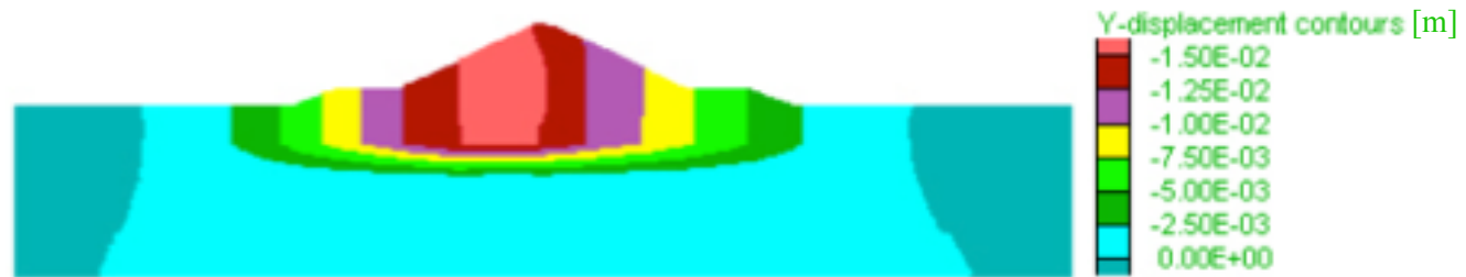
Vertical displacements [m] after the degradation of the first layer from GSI=80 to GSI=40
